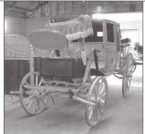
Colonial Williamsburg's 18th Century Wythe Chariot showing Thoroughbrace suspension and removable driver's seat
