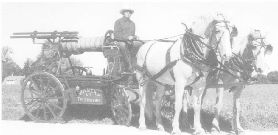
6-Man Pumper—Frank Tremel of West River, Maryland, is a breeder of American Cream draft horses, the fire chief of Engine No. 11 in Washington, D.C., and the owner of this hand pumper. Designed for use by a bucket brigade, it has a 100-gallon water tank and a 6-man hand pump. It was made in Vienna, Austria, and is one of only three such pumpers known to exist in the United States. Jack C. Norbeck, Coplay, PA
